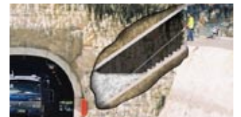
Such an access tunnel can be re-opened later, if required
