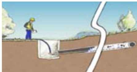
Pipelines inaccessible at one end are easily filled uphill or downhill
