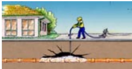
Benefil encapsulates a washaway section and restores support to the ground above
