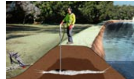
Sealing leaks in canal banks, levees and dams
