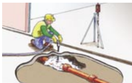
Washaways, compaction and subsidence frequently cause voids beneath factory floors
