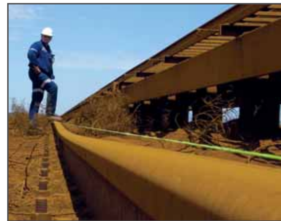
Below: Raising and re-levelling the slab restored proper engagement of the index machine gearing with the spline.
