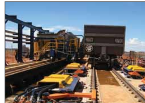
Below: Raising and re-levelling the slab restored proper engagement of the index machine gearing with the spline.
